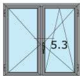
double sash window
